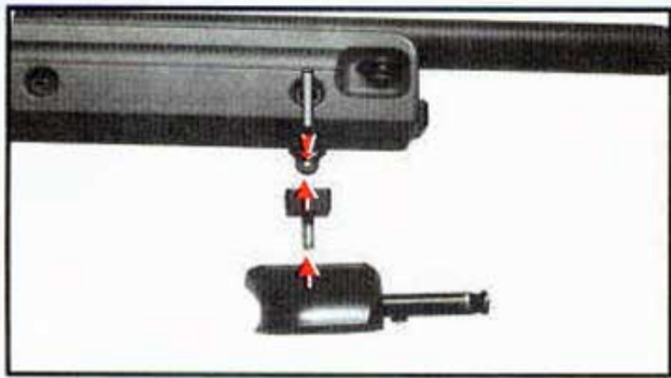
3. Install the horse as the arrowhead point. 安装脚架部件，按箭头所示。
