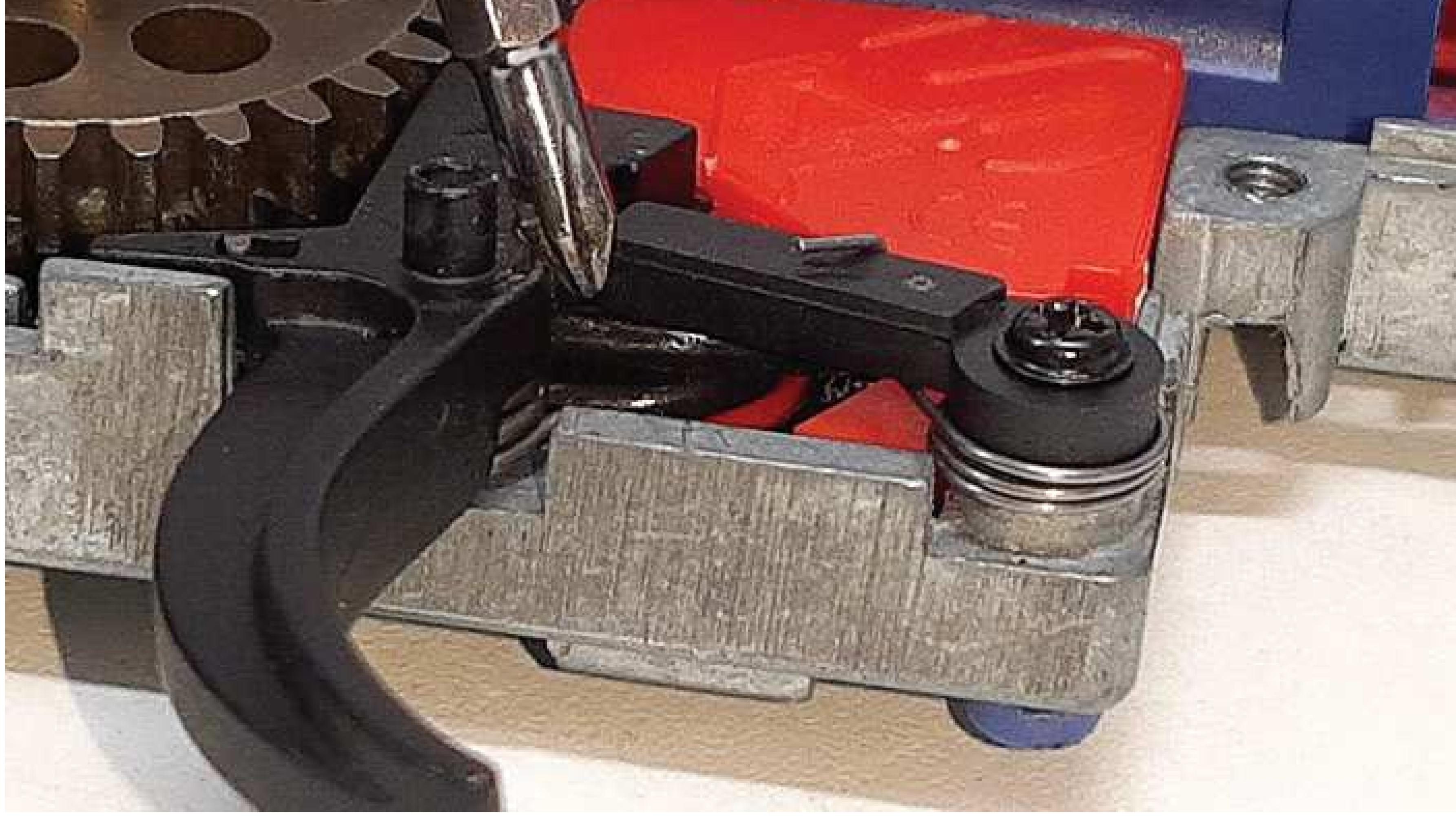
it has to moove freely. If needed change with the provided with the kit safety lever as it provides more clearence.
