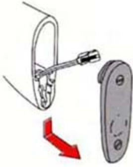
Remove the butt plate by pressing it downwards and pull out the connector.
