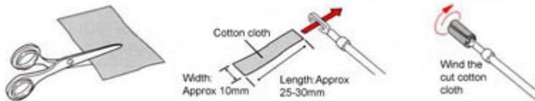
Cut the cotton to the size shown. Adjust the length accordingly so that it can be inserted smoothly into the barrel.
