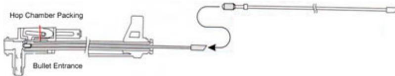
1. Apply a few drops of silicone from the bullet entrance, insert BB bullets into the magazine and fire bullets and fire bullets equivalent to 1 or 2 magazine.
