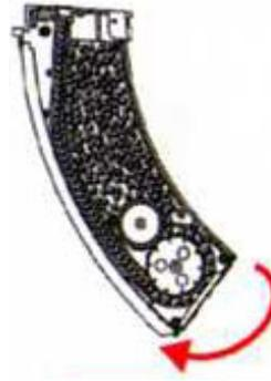
Move the gear with hand clockwise until it is fully wound, and the bullets will be sent up automatically (It can send about 150 rounds automatically)
