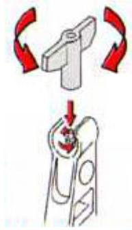
Insert the front sight adjustment tool in the front sight and turn it for adjustment.
