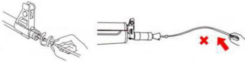
Hold at the leading end of the rod and insert the rod into the barrel while turning the rod.
