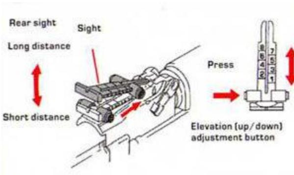
The 028 series rear sight is a tangent type which is adjusted vertically according to distance to the target.
