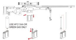
REPLACE THE MAGAZINE STRIP OR RELOAD BB DIRECTLY
