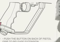
GRIP TO RELEASE EXTENSION · HOLD THE BUTTON DOWN TO ADJUST EXTENSION LENGTH
