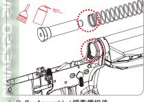
Clean all areas and out of fouling, Metal debris and dirt.
