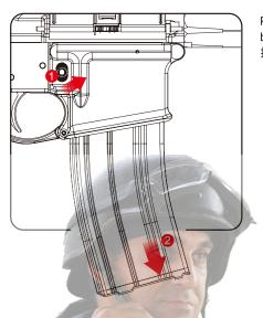
Press the magazine release button to remove the magazine. 按壓彈匣釋放鈕並卸除彈匣
