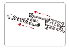
5.Remove the Bolt Assembly/卸除槍機組件 Pull back the charging handle.Take down the bolt carrier and bolt. 同後拉出槍機拉柄,並取出槍機。
