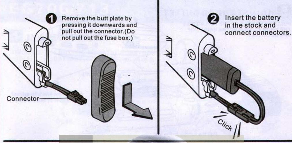
Press down the fuse box and insert connectors and cords between the fuse box and battery.
