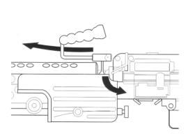
1 You can remove the outer barrel by lowering the lever.
