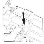
When removing the magazine, please use the thumb to push the button/magazine catch and pull it out slowly.
