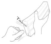
Check the BB pellets are lifted up to the exit, and then connect the magazine to the gun.
