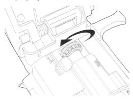
With hop up, BB pellets are able to extend its trajectory with revolution. Adjust with 2mm wrench.
