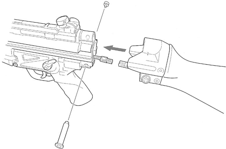
3 Take off the pin, then pull out the grip & gear box.
