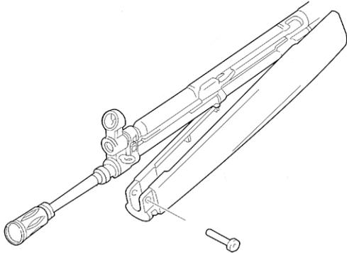
2 Take off the pin & pull out the stock. Be careful with the connector.
