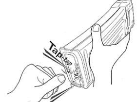
If pellet feeding is frequently in fault, remove all pellets from the magazine and spray silicone oil for 1 to 2 sec. Note that the hop-up operation may become unstable for a while after using silicone oil.
