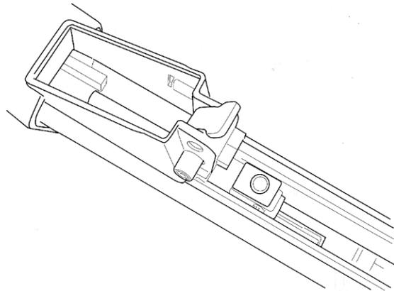
5 Pull the cocking lever for checking the hop-up chamber.
