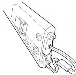
Insert the battery into the stock and connect the connectors
