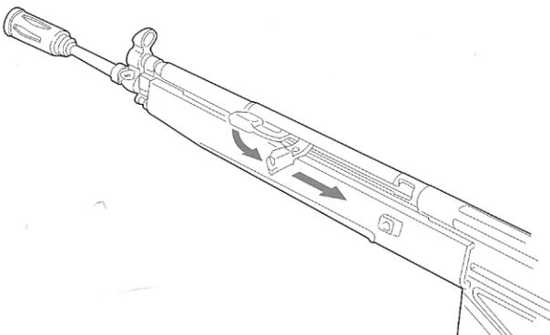
6 Use the sight adjustment tool to adjust the hop-up chamber.
