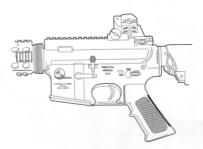
Separate the upper and lower receiver. Be careful of the wire
