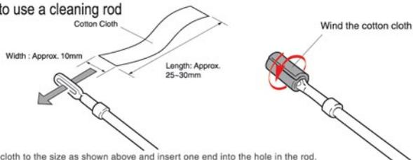
Cut a cotton cloth to the size as shown above and insert one end into the hole in the rod.
