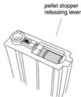
4. Hold the BB pellets entrance facing up and turn the gear at the bottom all the way until the click-click sounds change. (If only a small number of BB pellets are inserted, the gear merely makes blank turning.)
