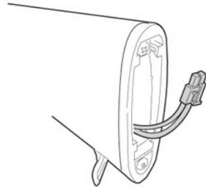
3. Insert the battery into the stock and connect the connectors.
