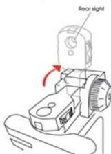
2. Turning the windage adjustment knob to adjust the precision firing
