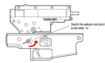
Slightly push the gear box into the body with your left hand,pry the body up with the screw driver, make sure the fan-shaped gear in the body is keep away from the selector gear on the gear box, and push the gear box into the body.
