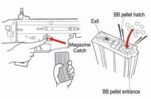
· Remove pellets remaining in the duct by reversing the magazine and using the release lever as shown. This ensures smooth operation next time.
