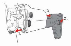
Insert the battery into the stock.
