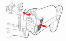
3 Take out the connector and connect it with the battery.
