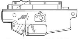
Make sure the fan-shaped gear in the body is totally matched with the selector gear on the gear box now.
