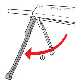
Press the switch then pull up the bipod
