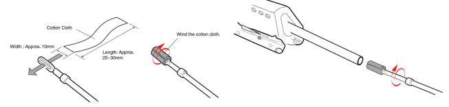
Cut a cotton cloth to the size as shown above and insert one end into the hole in the rod. (Adjust the length of cloth for smooth entry into the barrel.)
