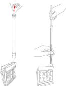
Press in bullets using the rod.
