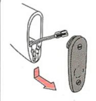
Remove the butt plate by pressing it downwards and pull out the connecter.
