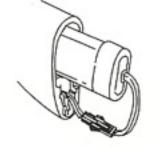
Insert the battery in the stock and connect connecters
