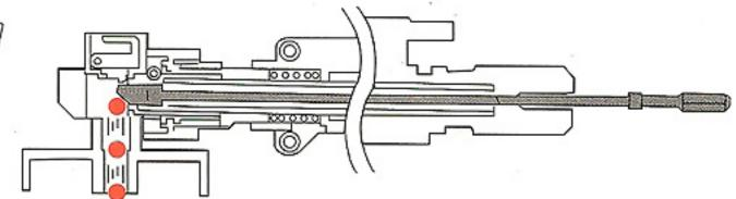
be careful so that the angled part of the cleaning rod faces down, and remove clogged bullets. 注意清彈器的尖角部分必須朝下,再取出塞滿的子彈。
