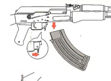
Press the magazine release to remove the magazine. (support the magazine as it may drop.)
