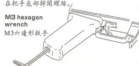
Insert M3 hexagon wrench into the screw hole to adjust. 將M3六邊形扳手插入螺絲孔里調整。
