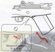
Press the release lever towards the trigger to lock.
