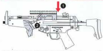
Insert the sight housing from above the gun until it snaps, and then fasten it with a screwdriver.
