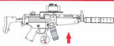
Make sure to set the magazine upwards and connect it firmly until a click sound is heard. 確保彈匣朝上并將其牢固地連接
