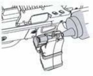
Move the gear with hand clockwise until it is fully wound, and the bullets will be sent up automatically. (It can send about 110 rounds automatically
