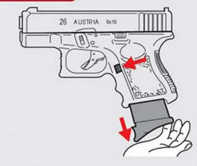
Attention: use hand to receive the magazine to prevent it from falling down to the ground.
