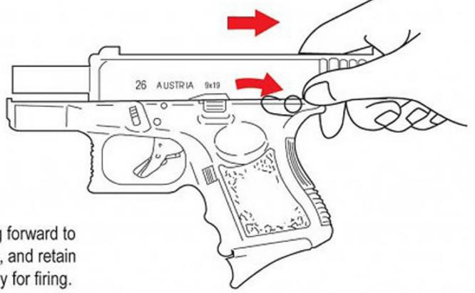
Then release and let the slide moving forward to load the pellet into the firing chamber, and retain the hammer at the rear position, ready for firing.
