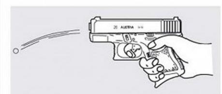
After a long and continued firing practice, the low temperature of the magazine will cause a reduced gas pressure as well as the low velocity of pellet. It is a normal condition and not a trouble.
