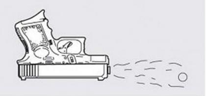
After the last BB pellet is fired, the slide will be retained in the back position, it means an empty magazine condition. If you want to resume the firing, insert a new fully loaded magazine; press the slide lock to release the slide and to reload the BB pellet.
