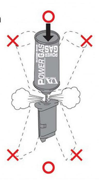
To refill the gas with the gas container in vertical position.
