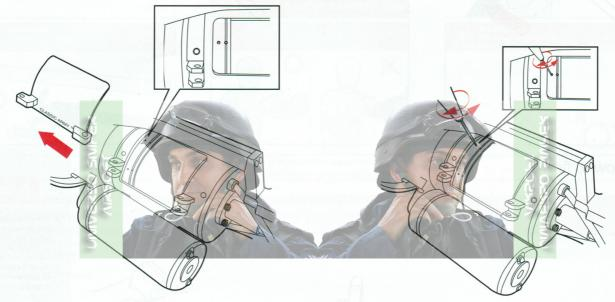
After adjustment turn the barrel to check if the dial is too loose.
