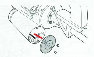
3 Connect the battery to the connector.
