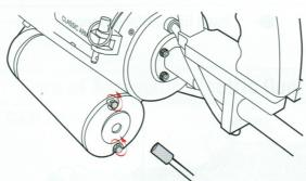
Press the trigger to test the rotation of the barrel. It should turn anti-clocwise.
