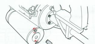
Remove the cover and pull out the connector.
