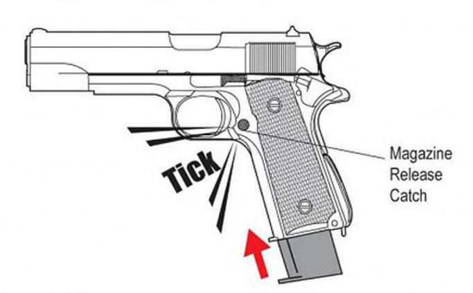
While loading the magazine, push it inward to the bottom till a "tick" sound is heard. Press the magazine release catch, the magazine will fall off from the stock.
