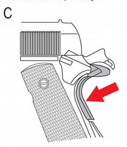
Grip Safety function can be applied automatically and grip the apron block tightly to release it.
