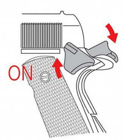
Hammer can only work when the safety switch stays at "OFF" position. Don't operate the trigger when the safety switch is at "ON" position. Otherwise, the pistol may be damaged.
