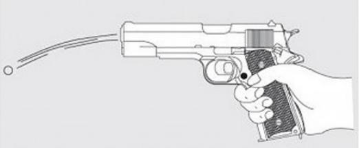
After a long and continued firing practice, the low temperature of the magazine will cause a reduced gas pressure as well as the low velocity of pellet. It is a normal condition and not a trouble. Never practice the reverse firing because which action causes the gas can not evaporate and the vaporized gas easy to damage the parts.
