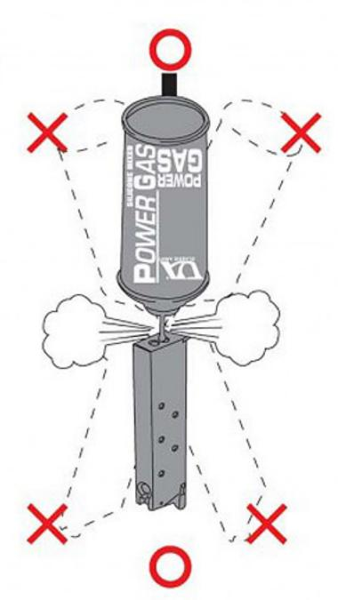
To refill the gas with the gas container in vertical position.
