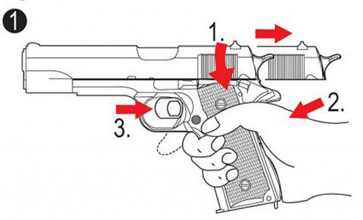
When the slide is pulled back and released forward. The BB pellet is loaded in the firing chamber, press the trigger to fire the loaded BB pellet.
