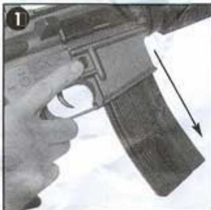
**1** To release the magazine, push on the magazine catch located on the side and slide the magazine out of the rifle. (Make sure the rifle is stored empty of any ammunition, magazine removed, and safety on).
