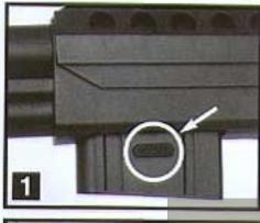
To remove the magazine, press the release at the same time on both sides of magazine and slide magazine out
