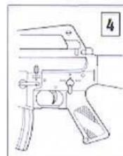
Since this is a single shot action rifle, the "Auto" and "Semi" positions do not make any difference in the firing mode. The rifle needs to be cocked after each shot.
