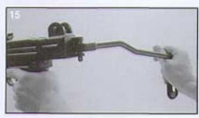
The stock is a folding type. To unfold it, push rear part of the butt to the right. To fold it, push it to the left.
