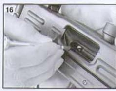
USER DISASSEMBLY 1/ Take off the bolt cover as shown on the picture.
