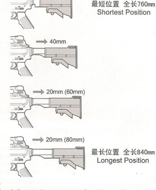
Pull it to the lock place, the lock controller . 2 4 can replace automatically and relock the gunstcok. 拉到某个锁定位置后,解锁控制杆会自动复 Click 咔哒 位, 重新锁定枪托.
