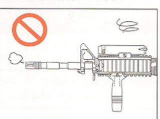
When bullets are clogged,immediately stop operation. Remove clogged bullets and then restart operation of the air gun.
