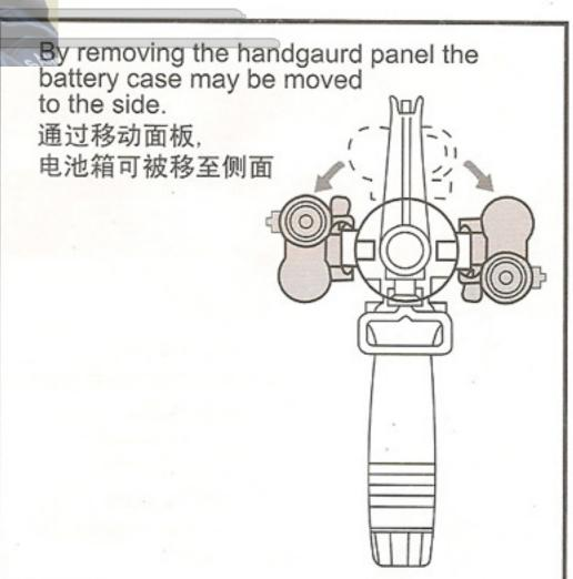
Removing the Battery Case 移动电池盒
