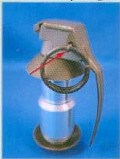
Install handle and safety key.
