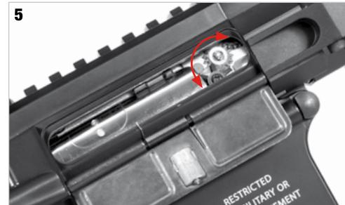
To adjust the Hop Up **turn the gear clockwise** to increase the effect and **counter-clockwise** to decrease it.
