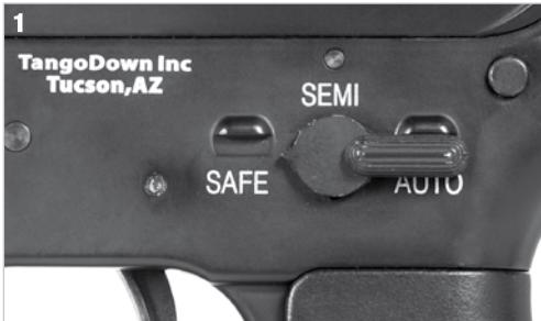
The selector lever allows **three positions**:
