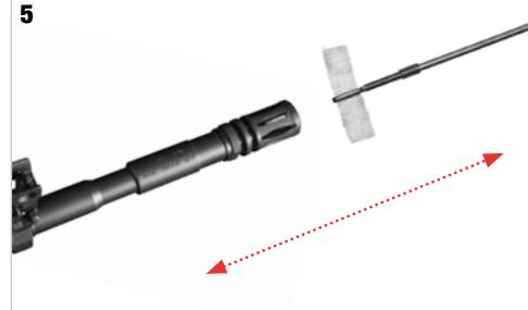
After **each use** always clean **the barrel** using the **cleaning rod provided** and a small piece of fabric, **soaked in silicone oil**.
