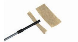
Cut the cloth or paper towel in the size as shown above. Fold the material to fit through the loop. Adjust the length of the material to smoothly enter the barrel, otherwise too much material will get jammed in the inner barrel and can cause the hop up bucking to get out of place.
