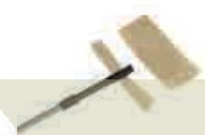
Cut the cloth or paper towel in the size as shown above. Fold the material to fit through the loop. Adjust the length of the material to smoothly enter the barrel. otherwise too much material will get jammed in the inner barrel and can cause the hop up bucking to get out of place.
