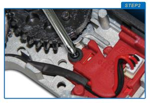
Remove the safety lever before install the E.T.U. Replace the trigger switch with G&G E.T.U, and tighten the screw.
