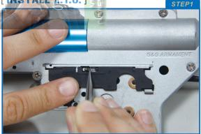
Remove the spring and selector plate. Replace the selector plate (included in the pack) for E.T.U. and install the spring.
