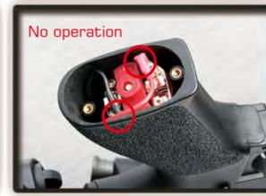
Check the wire set contact on the motor.
