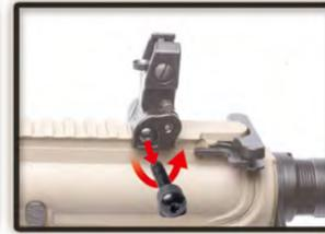
Remove the screw by turning counterclockwise.
