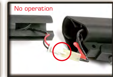
Check the battery and connector.
