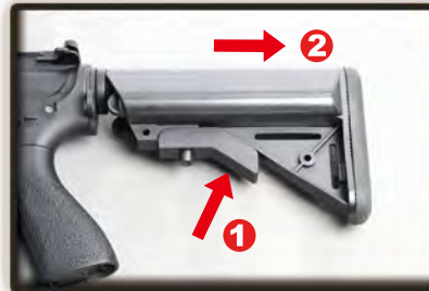
Press the stock release lever to unlock.
