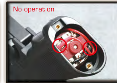
Check the wire set contact with motor.
