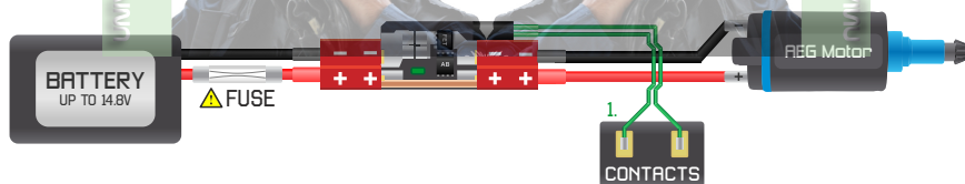
FIG 3. COMPLETE RE-WIRING SCHEME
