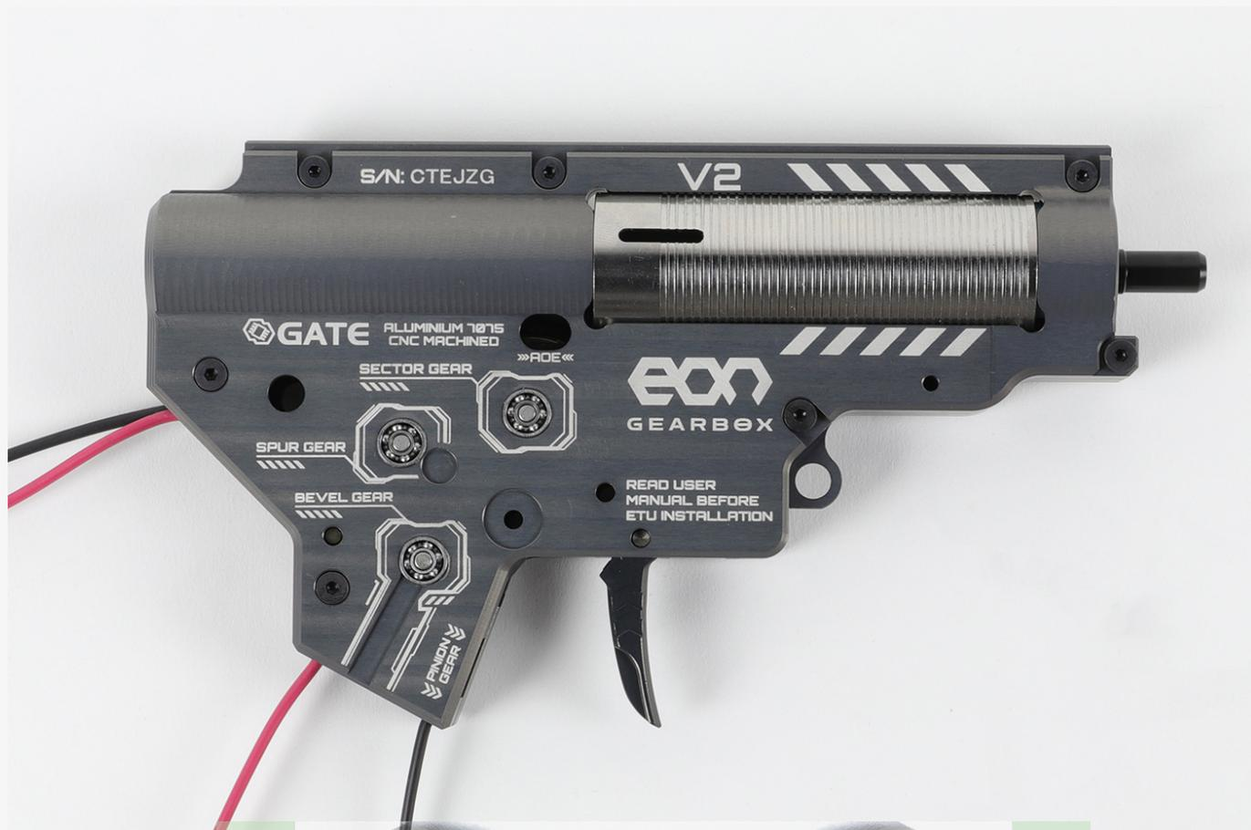
2. Open the gearbox and then remove the TOP TITAN II® board and plug-in the bolt-catch button into the multifunctional port.
