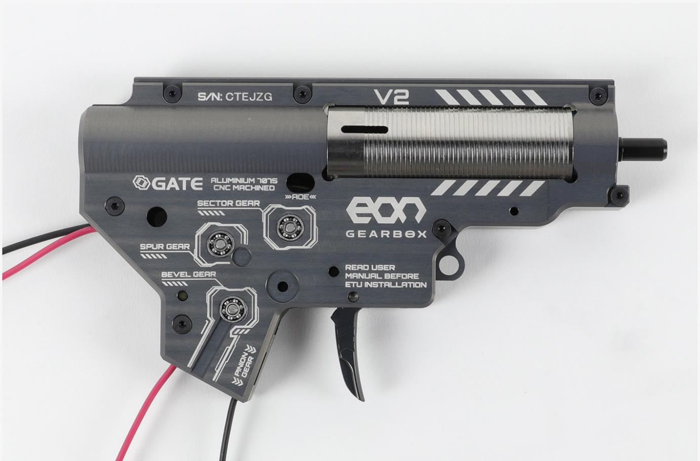
2. If possible, remove the piston spring before unscrewing the gearbox screws. Otherwise, unscrew the gearbox screws and carefully remove the cover making sure that the spring does not shoot out of the gearbox.
