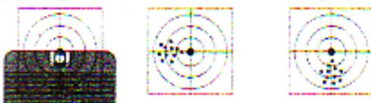
□ To aim the left, turn with a right-angled screwdriver the right screw on the rear sight rightward. It would be deflected to the left if rotate it leftward.
