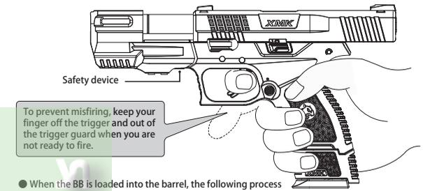
When the BB is loaded into the barrel, the following process will be proceeded and repeat automatically everytime you pull the trigger: BB fired → Slide movement (blowed backward) → Load the next BB (slide re-positioned)
