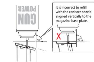
Please turn the magazine up side down to keep the injection hole side up, fill the gas only when the canister is verticalize to the injection hole. The gas will not be filled into the magazine or will leak out if the canister is not verticalized to the injection hole.
