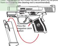
3 Press the slide catch lever to release the slide. ¶ Pull the trigger and fire several times towards safety directions, and make sure no BBs are left inside the barrel.
