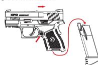
③ Push the slide catch lever upward to hold the slide at the rear. Turn the slide release button upward to head 12 O'clock direction, hold your slide with your hand then press the slide
