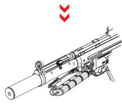
將電池接頭接好後再把護木固定 Plug in the battery and assemble the handguard.
