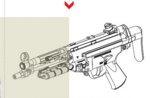
將電池接頭接好後再把護木固定 Plug in the battery and assemble the handguard.
