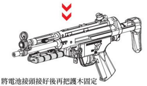
Plug in the battery and assemble the handguard.
