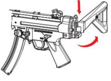
按壓槍托卡榫即可折疊 Push the butt catch and fold the stock
