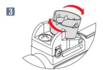
旋轉覘孔調整覘孔高度。 Turn the rear sight drum to adjust rear sight height.
