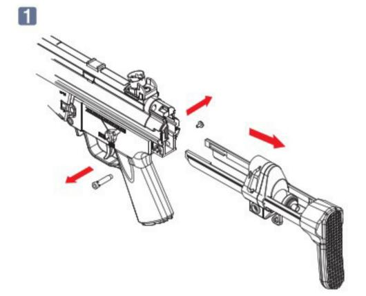
將槍身結合銷拉出後再把伸縮托整組拉出 Pull out the receiver pin Pull out the retractable stock.
