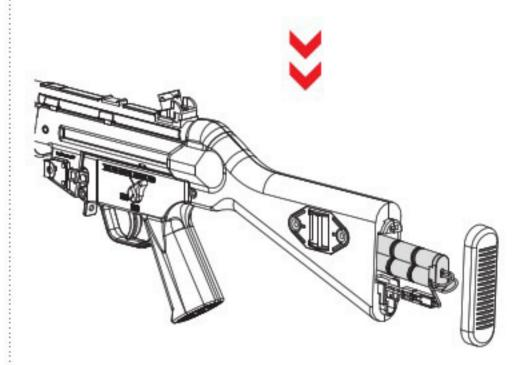
將電池接頭接好後放入槍托內再把槍托底板固定 Plug in the battery, put the battery into the fixed stock, and assemble the butt plate.
