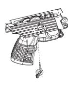
翻轉至另一側將選擇鈕卸下 Disassemble the Fire Selector on the opposite side
