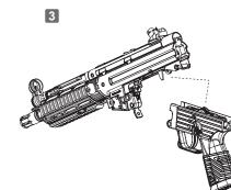
將後槍身結合銷取下後,再將槍托向後取下 Remove the stock by pulling out the rear receiver pin.
