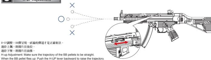
When the BB pellet flies up: Push the H-UP lever backward to raise the trajectory.
