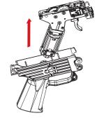
向上將下齒輪箱取出。 Pull up the lower gearbox to detach.
