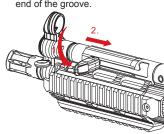
2 將槍機拉柄向上扳即可固定在後 Push the charging handle upward hold backward.
