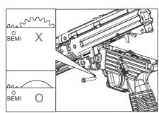
3號齒在槍身結合時,必須轉到正確位 置,才可將上槍身蓋下。 Make sure the sector gear is turned to the correct position before reassembling the receiver.
