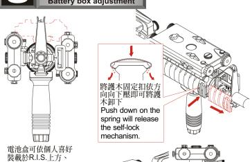
製献於R.I.S.上方、 左方或右方(如上圖) The battery box can be loded to the top, left, right as shown.
