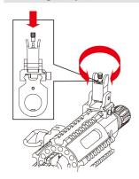
將準星調整桿壓入定位轉動 即可調整高低 Turn clockwise to raise B.B. hitting point. Turn counter clockwise to lower B.B. hitting point.
