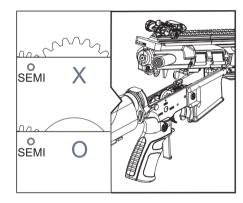
3號齒在槍身結合時,必須轉到正確位置, 才可將上槍身蓋下。Make sure No.3 gear is turned to the correct position before you reassemble the receiver/gearbox.
