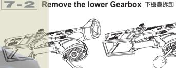
1 旋開馬達底蓋螺絲 Take out the screws on the plate.
