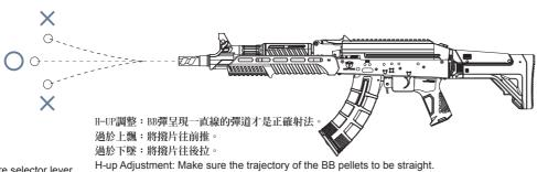
When the BB pellet flies up: Push the H-UP lever forward to lower the trajectory.
