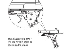
Install Gearbox into Receiver.
