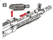
將上護木取出後,即可卸下彈簧。 Remove the upper handguard from the top, then remove the spring.
