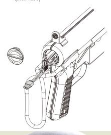
3 如為安裝鎳氫電池,請將其中的兩條 3 連裝電池以上下並排的方式置入電池倉的最底側 If installing the Ni-Mh battery, please put 2 sticks of 3 pcs connected battery down side by side into the bottom of the battery room.
