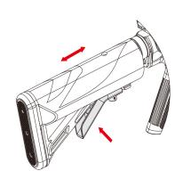
內壓即可調整伸縮托長度 Push the tab to adjust the length of retractable stock
