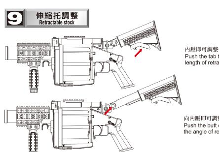
內壓即可調整伸縮托長度 Push the tab to adjust the length of retractable stock
