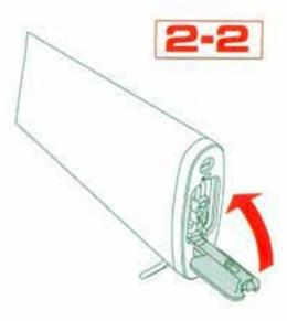
H.將電池與電線定位好,再蓋 上槍托底板蓋。 Place the connector in place and close the cover properly.
