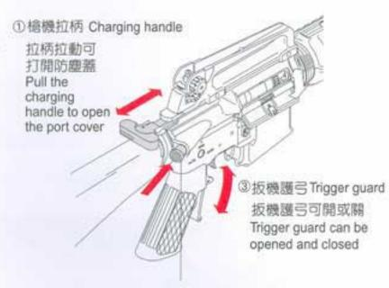
② 植機助進器 Forward assist knob 槍機助進器能夠推動 Forward assist knob can be pushed.
