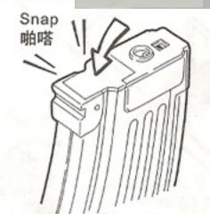
Slide the lever in the arrow direction to remove remaining BB bullets.(Be careful since BB bullets may jump out. 按箭頭方向滑動控製 杆, 取出射擊剩下的 BB彈(注意不能飛出)
