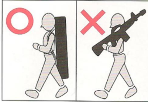
While carrying the soft ballistic gun, make sure the muzzle is tightly covered by the lid, and should be put in the bag or box.
