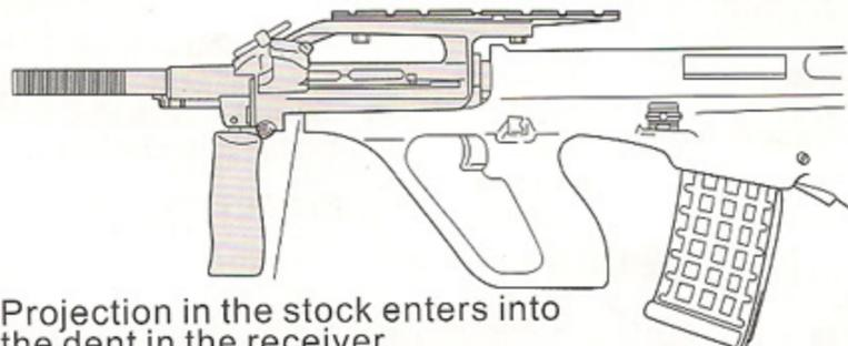
Projection in the stock enters into the dent in the receiver.
