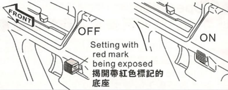
Always set the Safety to ON when you are not firing the gun or during storage. Also, put on the protective cap without fail. 當你不在射擊或收藏該槍時，請始終將保險裝置設置在打開位置。同時不要忘了系上保護帽。
