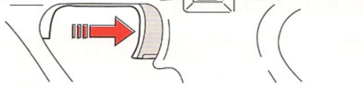
Semi Auto (Single shot) Pulling the trigger to the midway (about 4 mm) fires a single bullet.
