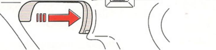
Full Auto (continuous Shooting) Pulling the trigger all the way (about 7mm) fires bullets continuously while you are pulling the trigger. Releasing the trigger slightly Stops firing.
