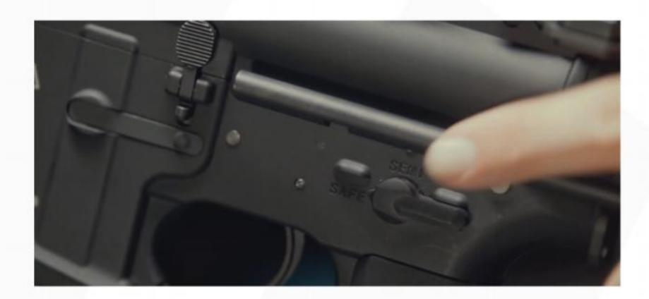
The selector which can be found on either side of the gun had 3 modes, safe, semi, and full auto. On safe, an internal mechanism will prevent the gun from firing. On semi, only one bb's will be shot out per trigger pull. On full auto, bb's will continue to be shot until the trigger is released. Once done firing always put the gun on safe.
