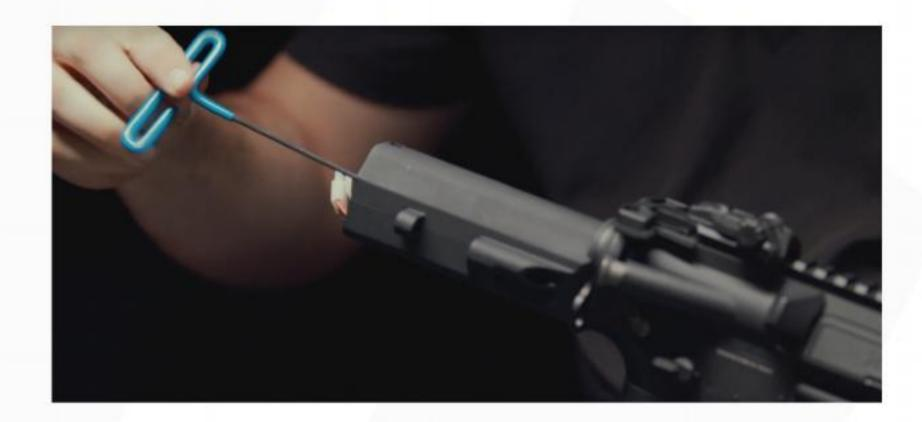
Twisting to the left results in less FPS, and twisting right results in more FPS. Once you have reached your desired FPS, reverse the process.
